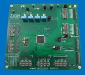
ADK-8475/6 → ARINC 429 Receiver with parallel and serial outputs Evaluation Board
